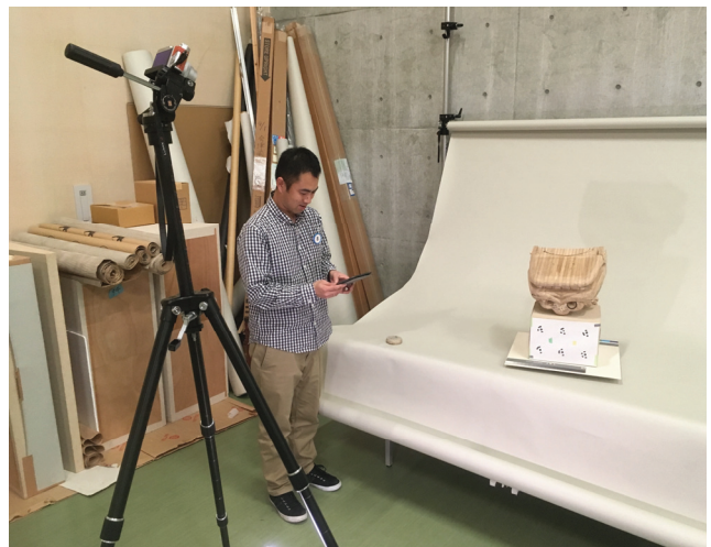
Fig. 2. Capturing images for Metashape processing using a tripod, a digital camera, and an iPad.
